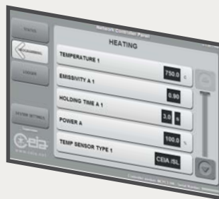
WEB SERVER & DATA LOGGER for remote service and quality control
